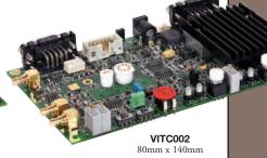
These Laser Diode Controllers are ideally suited for powering the expanded selection of Vertilas VCSEL diodes presented on pages 488 and 489. The Vertilas laser diodes can be plugged directly into the on-board sockets. Any other VCSEL diodes with grounded laser anode can be operated using a shielded DB9 cable.
