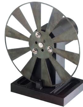
The MC1000A Optical Chopper, which includes a 10-slot (36°) chopper blade (MC1F10), is a precision instrument system utilizing advanced features to meet the most demanding applications. The MC1000A features a microprocessor control and a crystal stabilized phase-locked loop (PLL) motor control for ultimate chopping stability and drift-free performance.
