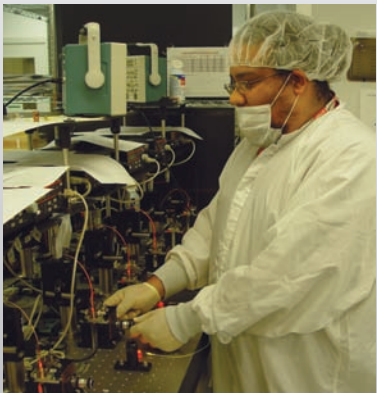
Pigtailed Laser Diode Alignment
