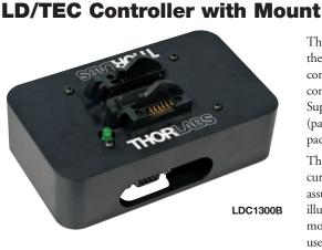
The LDC1300B Laser Diode Controller combines a laser driver, thermoelectric cooler (TEC) controller, and a butterfly mount into a compact package that can be controlled through an RS-232 interface. The controller is well suited for use with Fabry-Perot Lasers (pages 1249 - 1256), Superluminescent Diodes (pages 1356 - 1363), and Optical Amplifiers (pages 1367 - 1380) that have an integrated TEC in a 14-pin butterfly package.
