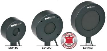
The ES100C series of general-purpose energy sensors can be used for detection in the 185 nm to 25  $\mu$ m range. A black coating on the sensor provides high, flat absorption over the spectrum, allowing it to measure energies from 3  $\mu$ J to 2 J. These sensors are available with an Ø11 mm, Ø20 mm, or Ø45 mm aperture. When using pyroelectric
