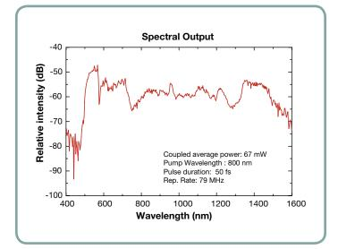
Dispersed Supercontinuum Generated with Coherent's Chameleon Ti:Sapphire Laser and the SCKB Supercontinuum Generation Kit.
