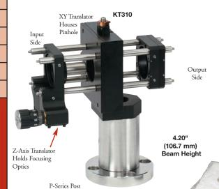
For many applications, such as holography, spatial intensity variations in the laser beam are unacceptable. Our KT310 spatial filter is ideal for producing a clean Gaussian beam. As shown in the photograph to the left, the input side consists of a Z-Axis Translator that will hold a diffraction-limited aspheric lens to focus incident light from a laser source through a pinhole. The pinhole should be mounted in the provided XY translator to allow easy adjustment.
