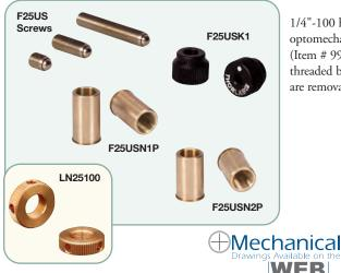
1/4"-100 hex adjusters are commonly used when making high-precision optomechanical mounts. Mating parts can be made using a tap (Item # 99940, see page 590) or with the F25USN1P or F25USN2P threaded bushings. Also available for use with the 1/4"-100 hex adjusters are removable knobs and vacuum-compatible ( $10^{\text{-}6}\,\text{Torr}$ ) lock nuts.
