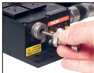
Removing the existing drive
