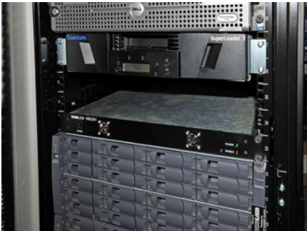
Click to Enlarge Figure 1.2 This image shows an RBD201 controller mounted in a typical 19" rack system.
