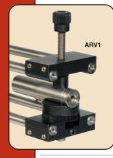
The cage clamps provide flexible adjustments within our 30mm cage assemblies. Both the top and bottom of the mount assembly can be independently translated along the Cage Assembly Rods while the base pedestals offer additional flexibility with lockable height and rotation adjustment. A top-located thumbscrew, complete with a swiveling Delrin<sup>TM</sup> tip, provides the fastening force required to hold securely optical components in place.
