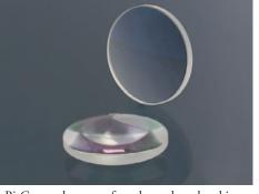
Bi-Convex lenses perfrom best when the object and image are on opposite sides of the lens and the ratio of the object to image distance (conjugate ratio) is between 0.2 to 5 or when used to create a virtual image from a real object.
