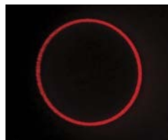
Fig 4: The photograph above shows the beam of a collimated laser beam after it is transmitted by an axicon.
