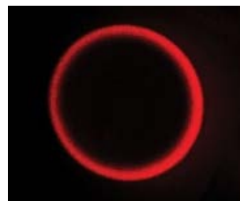
Fig 4: The photograph above shows the beam of a collimated laser beam after it is transmitted by an axicon.
