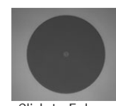
Click to Enlarge Undamaged Fiber End
