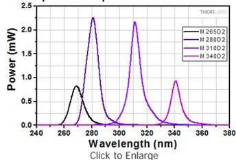
UV LED Spectra Scaled to Min Power
