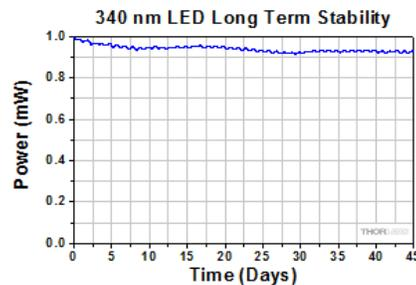
The M340L3 LED has a typical lifetime of >3,000 hours. In this case, the unit under test continued to provide more than 90% of its initial power after 45 days.
