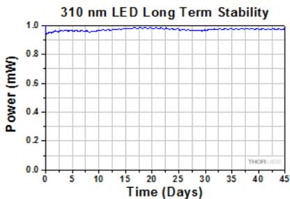
The M310L3 LED has a typical lifetime of >500 hours. In this case, the unit under test continued to provide more than 95% of its initial power after 45 days.
