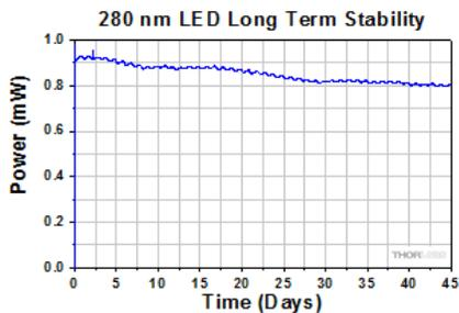
The M280L3 LED has a typical lifetime of >500 hours. In this case, the unit under test had dropped to ~80% of the initial output power after 45 days.
