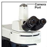
Click to Enlarge This microscope includes trinoculars with a 1X camera port for widefield viewing.
