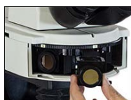
Click to Enlarge The rotating turret accommodates up to six filter cubes (not included).
