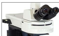
Click to Enlarge The CM2002 Cerna microscope features an epi-illuminator with a 6-cube filter turret. The filter position is labeled on the ring that rotates the turret. Three black sliders at the back of the housing contain neutral density filters.
