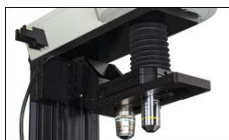
Click for Details 10X and 40X objectives (not included) mounted in the CM2002 microscope's dual objective nosepiece. The 10X objective is positioned in the optical path.
