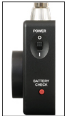
Click to Enlarge The Red Battery Test Button on the DET10D2
