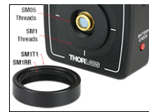
Click to Enlarge Each detector has an internal SM05 and external SM1 thread and comes with an attached SM1T1 Internal SM1 Adapter and SM1RR Retaining Ring.
