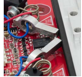
Click to Enlarge Red and blue wires deliver power to the motors, whose aluminum tips contact the black plastic strip at the edge of the linear stage.
