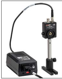
Click to Enlarge The PDA36A with the Included \pm 12 V Power Supply. Replacement power supplies are sold below.
