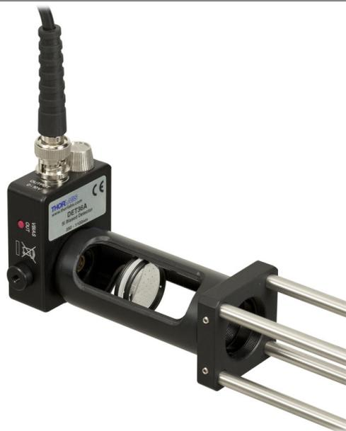
DET series photodetector mounted onto an SM1L30C  $\text{\O}1''$  Slotted Lens Tube, which is housing a focusing optic. The lens tube is attached to a 30 mm cage system via a CP02 SM1-Threaded 30 mm Cage Plate. This arrangement allows easy access for optic adjustment and signal alignment.
