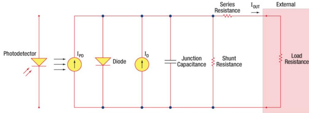
Figure 1: Photodiode Model
