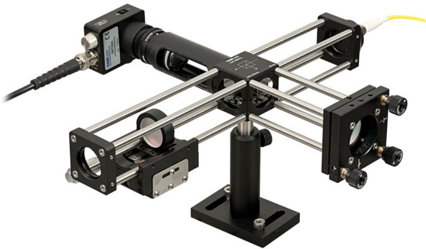
The table below contains a part list for the Michelson Interferometer for use in the visible range. Follow the links to the pages for more information about the individual parts.
