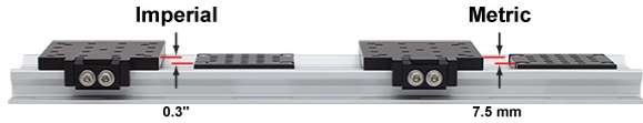
The difference between the mounting height of the imperial drop-on rail carriage and the imperial rail plate is 0.3" (7.6 mm). For the metric parts, the height difference is 7.5 mm (0.29").
