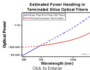
Plot showing approximate input power that can be incident on a single mode silica optical fiber with a termination. Each line shows the estimated power level due to a specific damage mechanism. The maximum power handling is limited by the lowest power level from all relevant damage mechanisms (indicated by a solid line).
