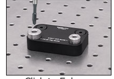
Click to Enlarge Once the TTT001(M) guide is properly aligned over the hole, use the TW25 Hand Tap Wrench with a 1/4"-20 tap (Item # 71598) or an M6 tap (Item # 71498) to restore the threads.
