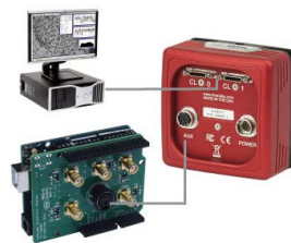
Click for Details A schematic showing a TSI-IOBOB2 connected to an Arduino in a custom camera system.
