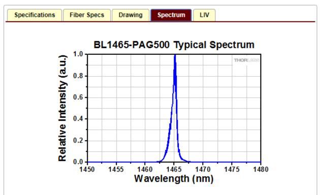
The typical optical spectrum is shown above. The laser diode was driven at  $P_{OP}$  (500 mW) and held at 25 °C. Performance will vary between individual lasers, serial-number-specific documentation is provided with each FBG-stabilized laser diode.
