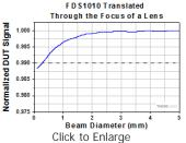
Figure 1: Normalized change in output current for a fixed incident power as the photodiode Device Under Test (DUT), FDS1010, was translated through the focus of
