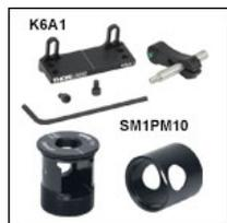
The K6A1(M) is a 0.5" x 1.44" platform designed to be mounted on the rotation ring of the CRM1T(M), CRM1LT(M), and CRM1P(M) 30 mm cage compatible rotation mounts featured above and the K6X six-axis kinematic mount. The K6A1 comes with a PM3 Small Clamping Arm (K6A1/M comes with PM3/M), hex key, and mounting screws. The K6A1 and K6A1/M have 6-32 and M4 x 0.7 tapped holes, respectively, on the mounting platform to secure the supplied clamping arm.
