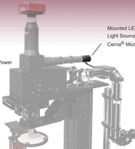
Mounted LED used as a Light Source for a DIY Cerna® Microscope
