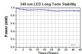
Our 340 nm mounted LED has a typical lifetime of  $>3,000$  hours. In this case, the unit under test continued to provide more than 90% of its initial power after 45 days.
