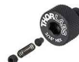
(1.5 mm) balldriver. The spring and tip can then be removed from the thumbscrew, in the order shown in the image to the right. However, the resulting contact face of the thumbscrew will have a center hole, unlike the contact face of our vacuum-compatible thumbscrews.
