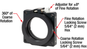
Click to Enlarge This mount offers 360° of coarse rotation via the rotation ring and ±8° of fine rotation via the threaded adjuster. The coarse and fine rotation are independent of each other and both positions can be locked using the respective 5/64" (2 mm) hex locking screws.
