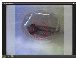
A predefined circle scan pattern can be loaded and scanned in the software. The size can be changed with the Zoom feature.
