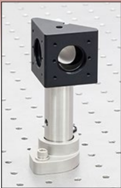
Application Idea Using an RBP1 Pin-Aligned, Clamping Post Base and KCB1 Mount to Align a Laser Above the Holes in an Optical Table
