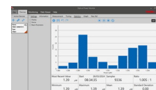
Click to Enlarge Figure 149C Power Statistics Mode Calculate numerical statistics for a pre-determined measurement period. The panel displays the analyzed values in a bar graph and the results as numerical values.
