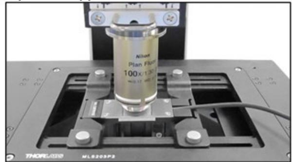
S170C Microscope Slide Power Meter Sensor used with a 1.30 NA Objective and Shown on an MLS203-1 Motorized Scanning Stage Equipped with an MLS203P2 Slide Holder
