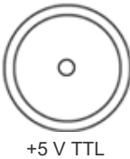
TRIG 1 (Defaulted to Trig In) SMA Female TRIG 2 (Defaulted to Trig Out) SMA Female
