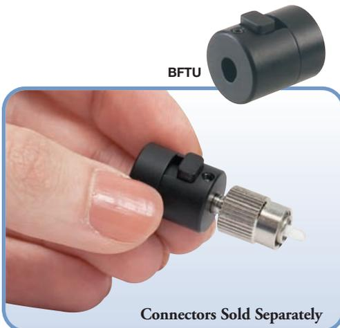
For applications where a temporary fiber termination is desired, our Bare Fiber Terminator is the solution. It is reusable and can be easily cleaned if the fiber breaks inside the connector by using the WC100 clean out wires (below). The bare fiber terminator is designed to mechanically hold fibers in standard connectors (sold separately). The BFTU accepts ferrules up to Ø0.158" (Ø4 mm) and fibers up to Ø0.03" (Ø0.7 mm).
