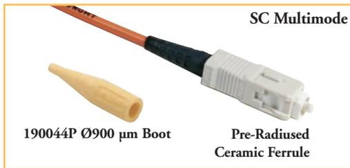
This SC-style connector features a pre-radiused (20 mm) ceramic ferrule that is packaged with a Ø3 mm boot and minimizes back reflections. The connector has a bore size of Ø125 µm. Each connector package includes a fiber connector cap and a Ø3 mm boot.
