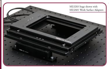
The MLSA01 Brackets enable the MLS203-1 XY Microscopy Stage to be bolted to an optical table or breadboard, thereby facilitating the use of this stage in custom-built microscope setups or general photonics applications. The brackets, which are sold as a set of two, fit both imperial and metric mounting surfaces. Please note that these brackets are not compatible with the MLS203-2 Microscopy Stage.
