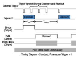
**Figure 2:** Asynchronous triggered acquisition mode. When the external trigger signal goes low, an exposure begins for the preset time, and then the exposure is read out of the camera. During the readout time, the external trigger is ignored. Once a single readout is complete, the camera will begin the next exposure only when the external trigger signal goes low.
