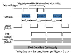
**Figure 1:** Streaming overlapped exposure mode. When the external trigger goes low, the exposure begins, and continues for the software-selected exposure time, followed by the readout. This sequence then repeats at the set time interval. Subsequent external triggers are ignored until the camera operation is halted.
