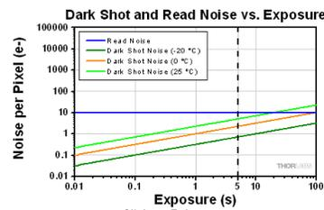
**Figure 1:** Plot of dark shot noise and read noise as a function of exposure for three sensor temperatures for our 1.4 megapixel cameras. This plot uses logarithmic scales for both axes. The dotted vertical line at 5 s indicates the values calculated as the example in the text.
