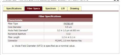
FPL785P-200 - 785 nm, 200 mW, Butterfly Laser Diode, PM Fiber, FC/APC
