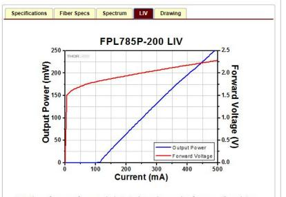
Note: the performance of one sample device is shown above, and performance will vary between individual lasers. Serial-number-specific documentation is available by clicking "Choose Item" on the left side of the price box. The device was held at 25 °C.
