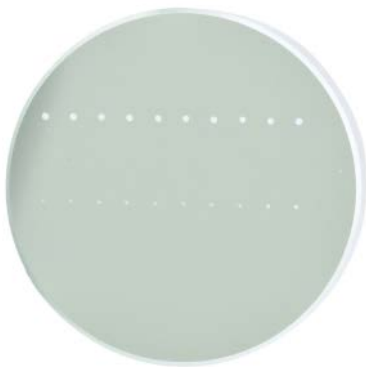
The photograph above is a protected aluminum-coated mirror after LIDT testing. In this particular test, it handled 0.43 J/cm 2 (1064 nm, 10 ns pulse, 10
