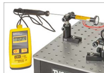
Figure 6. One mirror of the interferometer is mounted on the end of an aluminum rod that is wrapped in a heater. The rod temperature is monitored, allowing the coefficient of thermal expansion to be calculated using the temperature change and total number of fringes that move out of the center of the interference pattern as the rod expands.
