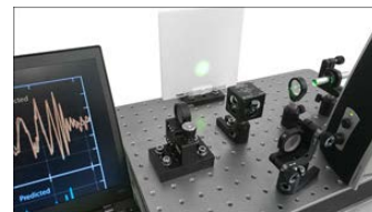
Click to Enlarge Loud music with a strong bass line causes fluctuations in the interference pattern.
