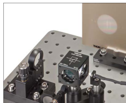
Click to Enlarge White Light Interference Generated with the Michelson Interferometer Educational Kit
