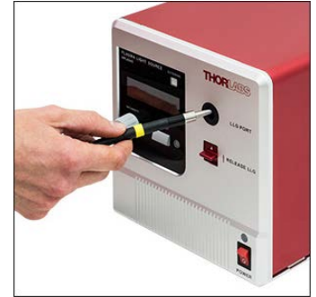
Figure 1: After ensuring the tip closest to the yellow band is clean, slide that tip into the LLG Port. Continue to push the end of the LLG into the port until the edge of the yellow band is flush with the front panel (Figure 2).
