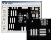
The screen captures to the right and left are actual measurements taken using a USAF 1951 resolution chart as the object.
