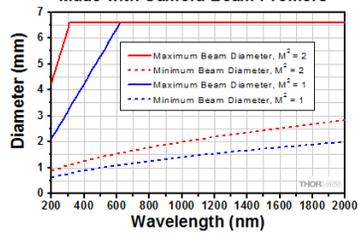
The range of beam diameters at the input lens that can be analyzed by the M<sup>2</sup> measurement systems for two cases: M<sup>2</sup> = 1 and M<sup>2</sup> = 2 are limited by the wavelength-dependent bounds plotted above.
