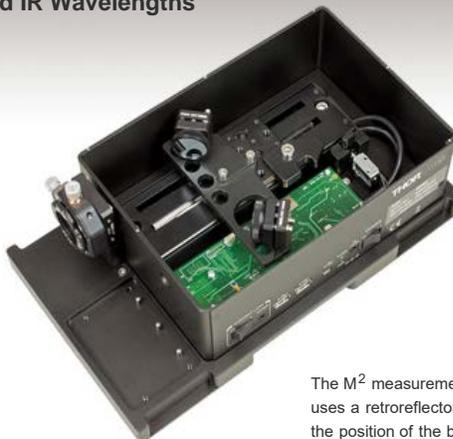
The M<sup>2</sup> measurement system uses a retroreflector to change the position of the beam waist with respect to the beam profiler.
