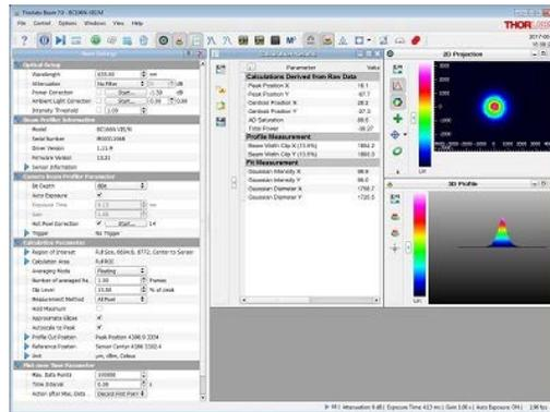
The main window of the GUI includes the menu bar, tool bar, status bar, and a frame where several windows can be displayed. This view includes a Beam Settings Panel that displays all important information in a single location and can be unpinned from the main window and moved to a second location, such as another monitor.
