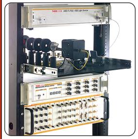
These slideout rack boards (1/4"-20 on 1" centers or M6 x 1.0 on 25 mm centers) allow optical systems to be built within instrumentation racks.
