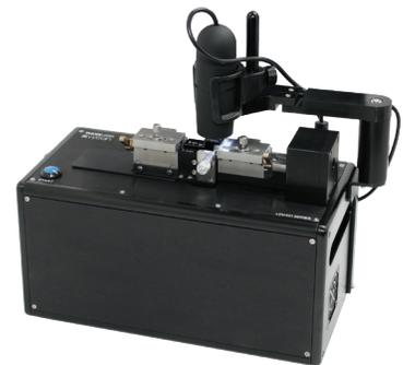
Our digital microscope kits allow the user to image the fiber, cleave blade, and micrometer position during the cleaving process.
