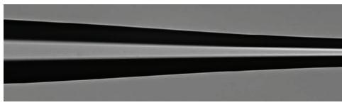
$\varnothing$ 20  $\mu$ m Core,  $\varnothing$ 400  $\mu$ m Cladding Large-Mode-Area (LMA) Fiber Tapered to  $\varnothing$ 125  $\mu$ m Cladding
