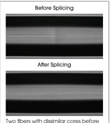
and after splicing. The dissimilar cores are clearly visible before the cores are thermally expanded.
