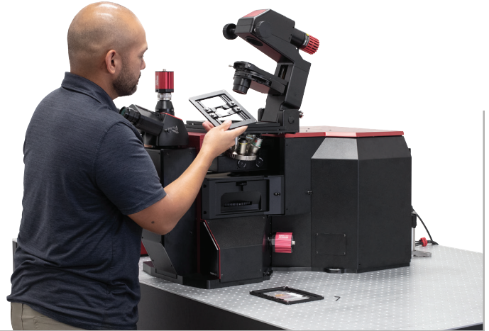
The MLS203 stage has many slide holders and accessory plates that are easily swappable.
